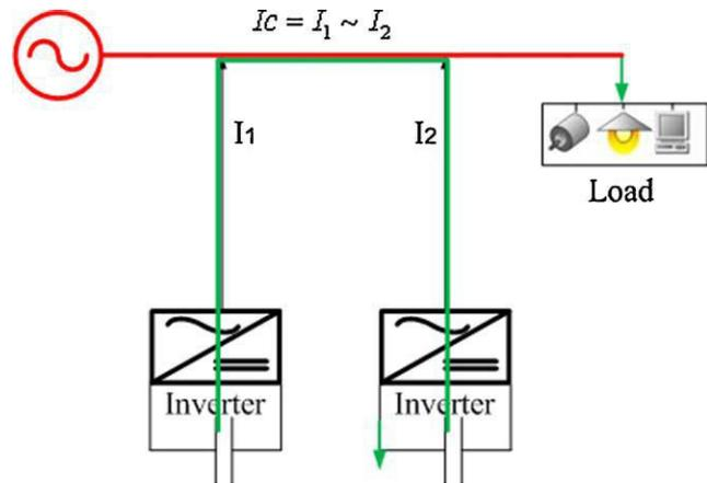
Fig. 2. Circulating current flow between the parallel inverters.
