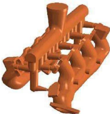
Fig(3.1) Mould tree assembly
